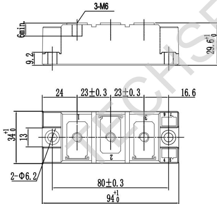
Unmarked dimensional tolerance: ±0.5mm
