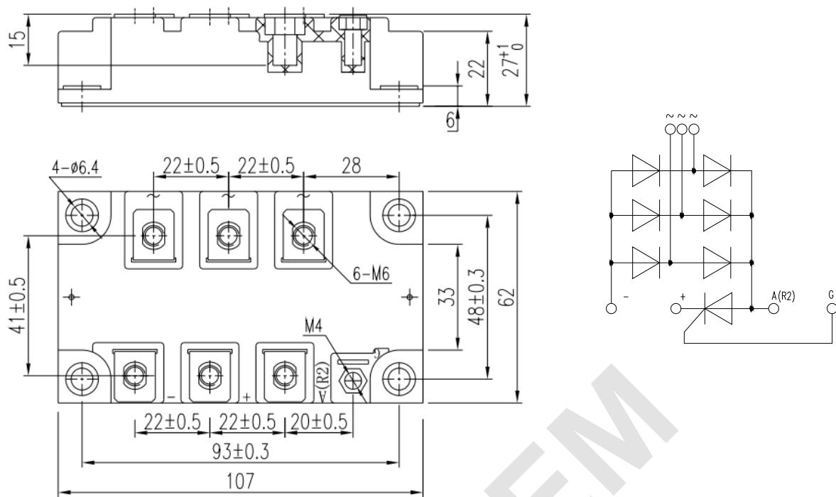
Unmarked dimensional tolerance:  $\pm 0.5\text{mm}$
